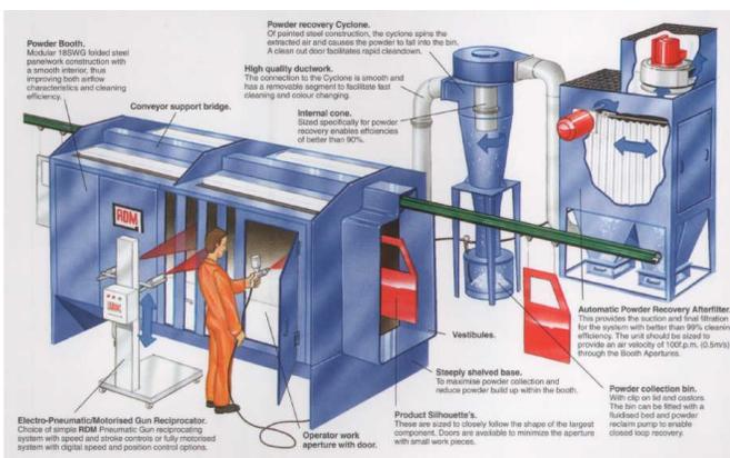
Figure 1.2 Powder Booth Schematic Layout
