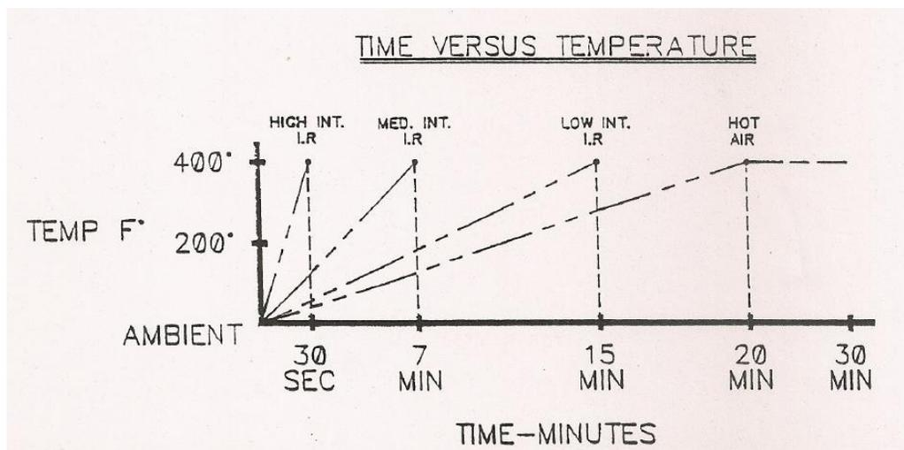
Figure 5.2 Comparison of product heat up rate of Short/Medium/Long wave IR and Hot air (BKG Finishing Systems)
