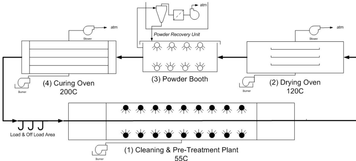
Figure 1.1 Powder Coat Plant Schematic Layout
