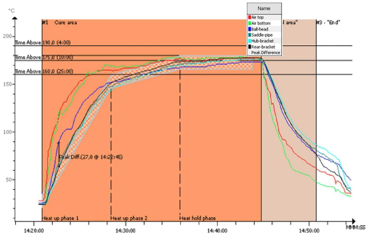
Figure 2.1 Temperature profile of curing a bicycle frame
