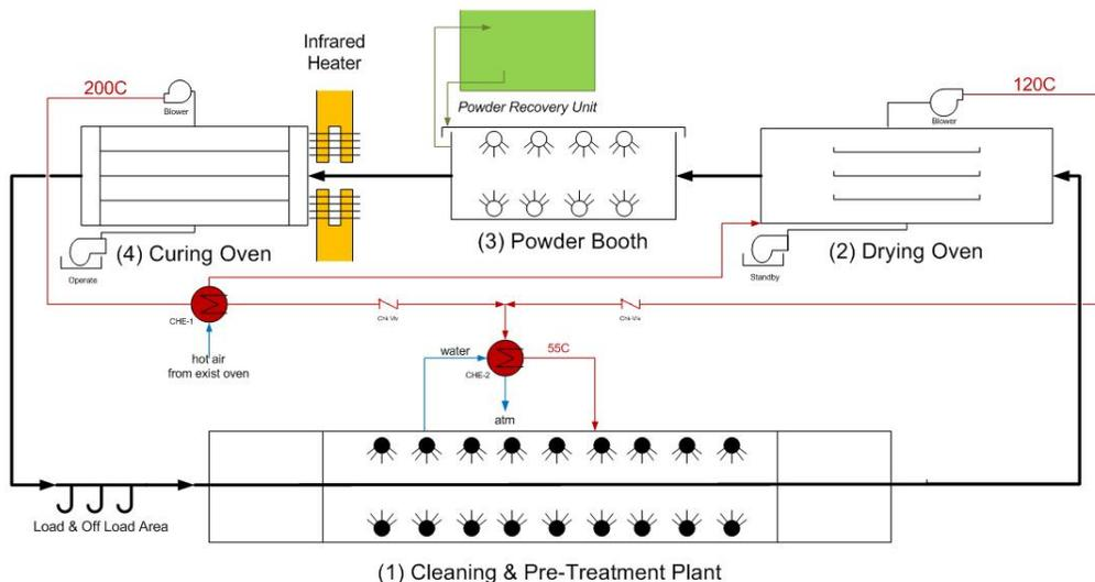
Figure 5.1 Conceptual Designs for new Powder Coating Plant
