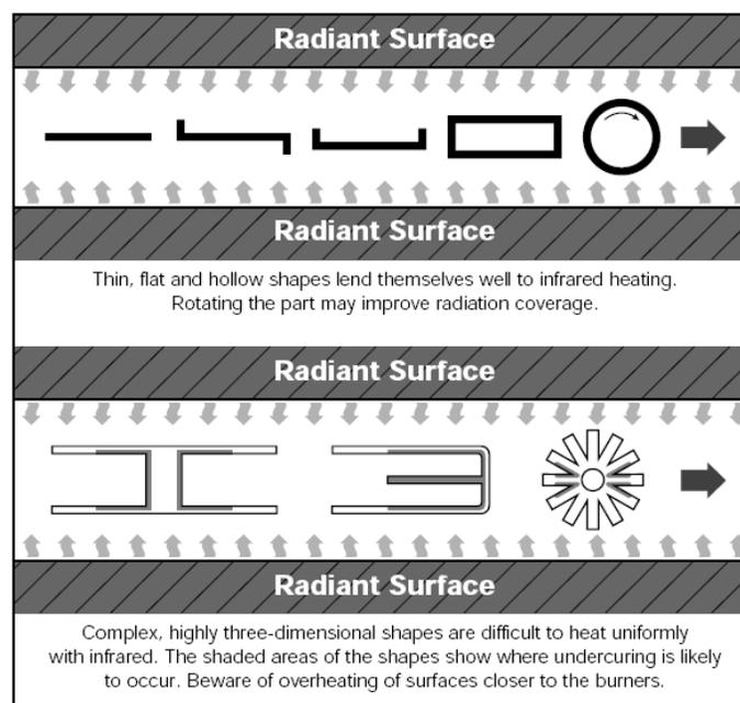
Figure 6.1 Suitable product configurations for IR heating (Eclipses Combustion)
