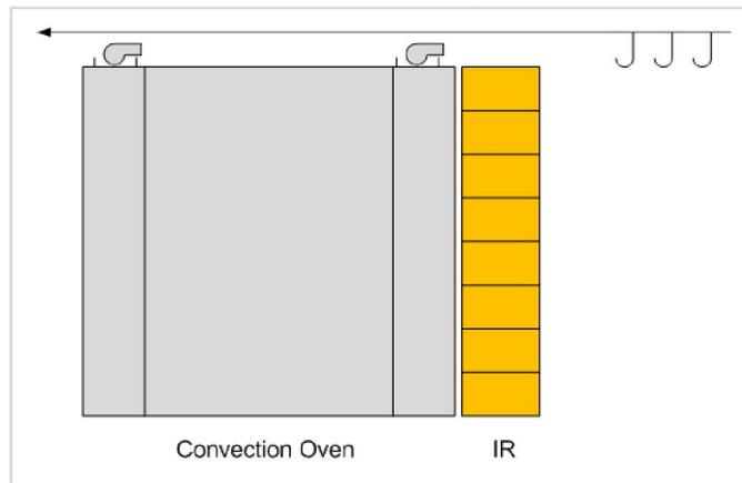
Figure 5.4 Combination oven (Convection + IR)
