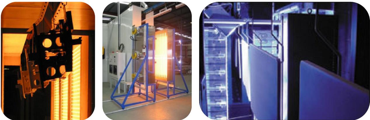
Figure 6.2 from left to right, IR oven, Combined IR/Convection oven and Combined IR/UV oven
